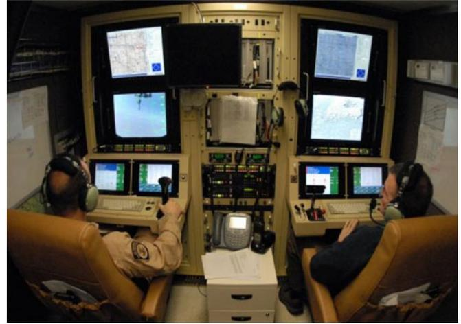
Fig. 3. Example of a MALE UAS *Mission Specialist* (Right) interacting with a General Atomics Predator UAV (Courtesy of United States Department of Defense).
